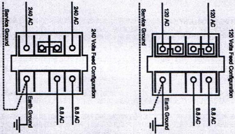
Power-On Transformer is shipped with primary windings configured for 240 Volts AC. Configure jumper straps according with electrical feed service. Grounding for transformer should be from service feed only. If service ground is not available within instrument housing, then use earth ground. This note does not supersede company policy and/or instructions.
